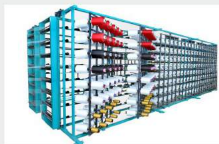
Cone Creel Swivel Frame Type Creel Ends : 320 to 1200 Creel Pitch : 240/280/350
