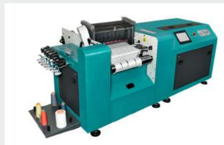
Sample Rapier Weaving Machine (50 cm / 5-30 meter / 8 colours)
